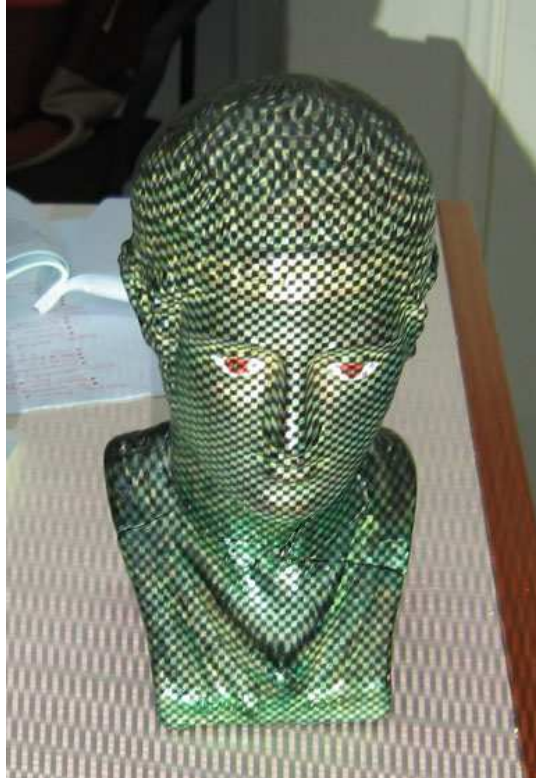
Figure 4.11: Projecting a pattern on the object we want to reconstruct creates additional feature points
